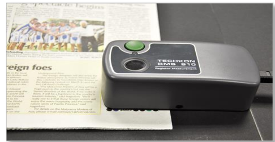
"Techkon spectrodens color measuring instrument (left) and Techkon "RMS 910" register measuring instrument (right)
